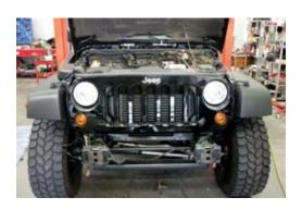
3. Remove fog lights from factory bumper bar and install to bull bar as shown. If winch is being installed, refer to winch installation instructions pages 4-7.
