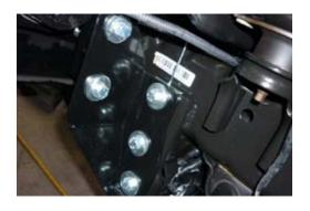
9. Align bull bar with vehicle and tighten all bolts.
