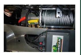
13. Connect the thin black earth wire and negative battery cable to the earth connection on the opposite side of winch motor.
