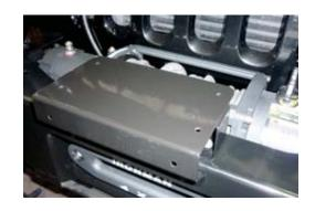
11. Place control box on control box bracket and mark four mounting holes.
