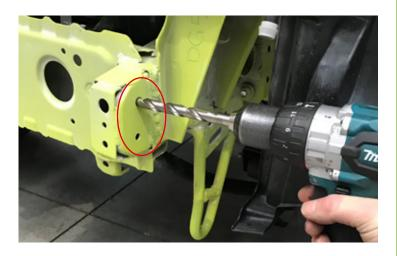
**4.** Drill 12mm hole on each side of the support beam as shown.
