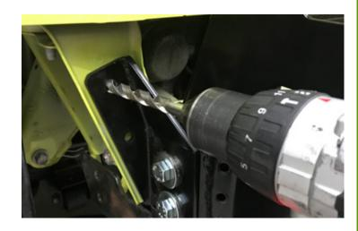
10. Insert support bracket into body mount area and attach using 40mm M10 bolts.
