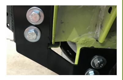
**9.** Using the support bracket as a guide, Drill two (2) 10mm holes through panel as shown.
