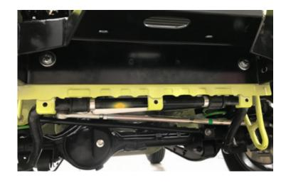
crush tubes and the remaining 75mm M12 bolts, washers, spring washers and nuts, sandwich the support beam through the two (2) centre holes of the cradle.
