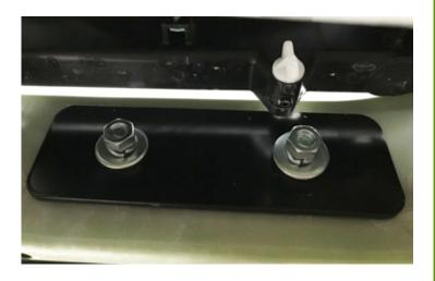
7. On the passenger side, use the bent support brace and attach to the two (2) outer holes of the cradle using two (2) 90mm M12 bolts, washers and nuts. (Use 24mm outside diameter washers on the inside of the cradle).
