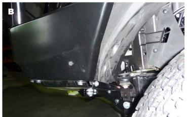
**34.** Fit protection plates to underneath of bull bar using M8 bolts, spring washers and flat washers provided.
