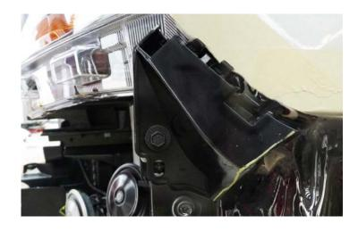
**9.** Remove air duct shields as shown. Disconnect temperature sensor from passenger side before removing.
