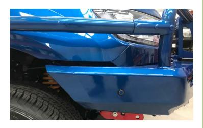
**31.** Once bar is aligned with vehicle and tighened, drill through pinning holes between bull bar and chassis bracket and secure with bolts, washers and nuts provided.
