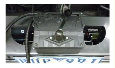
**4.** Connect three colour coded cables to the corresponding poles on winch motor.
