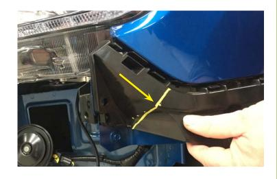
7. Mask lower edge of guard and paint lower section satin black as shown.
