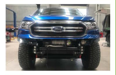
**6.** Using end of bumper bar as a guide, mark cut lines onto plastic bumper support brackets.
