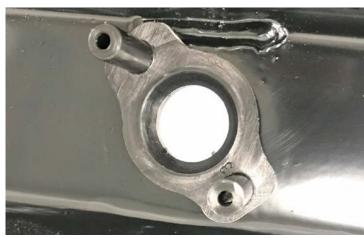
23. Remove bezel from parking sensors. The two outer wing parking sensors will require the extra '0' ring placed over the silicone sleeve.
