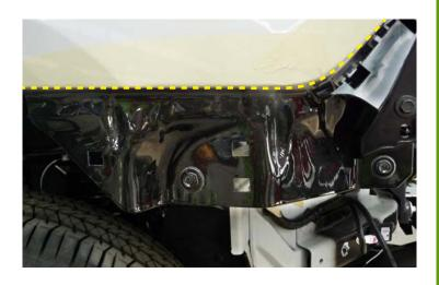
**8.** Re-fit plactic bumper bar support brackets as shown.
