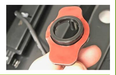
**22.** Remove the double sided stickers protective layer and install the sensor holder into the bar.
