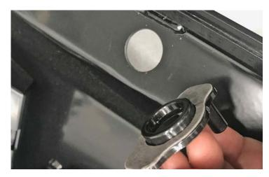
**IMPORTANT:** Parking sensors should be installed as close to the same direction as when they sit in the factory bumper.
