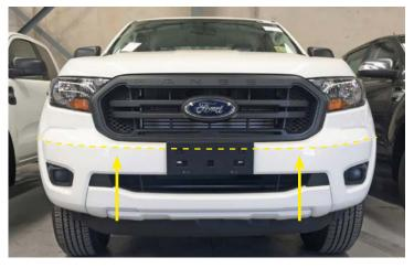
3. Disconnect and remove Adaptive Cruise Control from metal bumper support.
