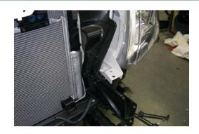
5. Remove plastic mud guard clips from lower mud guard lips.
