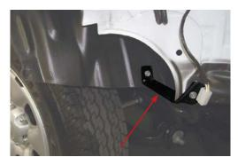
Note: Secure using a modified original lower bumper support bracket as shown.
