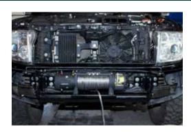
2. Bolt winch to cradle with gearbox to the left hand side of vehicle and cable spooling from bottom of the cable drum using bolts and washers provided.
