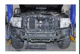
9. Cut bumper bar to remove lower section.
