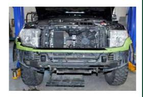
10. If winch is being installed, remove section of bumper bracket as marked in photo
