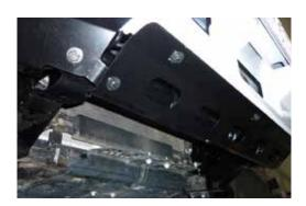
20. Trim guard liners and secure to radiator support panel with bolts and washers as shown.
