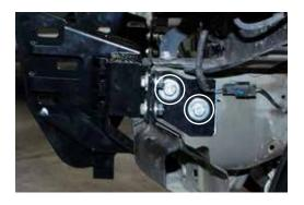
13. Re-fit top section of bumper bar and cut flares as shown. Install pinchweld.
