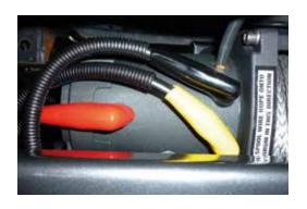
7. Connect the thin black earth wire and negative battery cable to the earth connection on the opposite side of winch motor.
