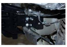
12. Using strengthening brackets as a guide, drill through sub frame and secure in place using long bolts, washers and nuts provided and tighten all mounting hardware.
