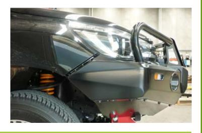
10. Once bull bar is aligned with vehicle and tightened, drill through pinning holes (circled in red) between bull bar and chassis bracket and secure with bolts, washers and nuts provided.
