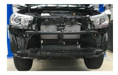
**3.** Fit inner and outer chassis support brackets with supplied hardware.
