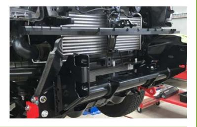
**5.** Cut plastic air-deflectors along lines as shown to allow fitment of bull bar to bracket.
