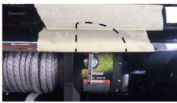
9. Fit bull bar to chassis brackets using M12 bolts, flat washers, spring washers and nuts provided. Align with mudguard leaving a 10-15mm gap as shown.
