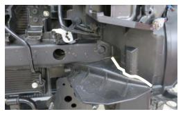
4. Fit mounting bracket with hardware supplied.
