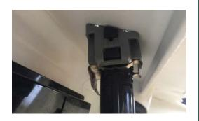
5. Lift squirters out of washer, remove and swap sides of grey nozzles to align spirters at headlight.
