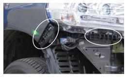
3. Cut plastic air-deflectors along lines as shown to allow fitment of bull bar to bracket
