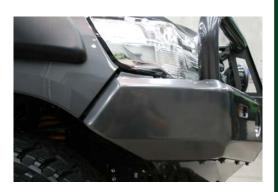
9. Once bull bar is aligned with vehicle and tightened, drill through pinning holes (circled in yellow) between bull bar and chassis bracket and secure the M-10 bolts, washers and nuts provided.
